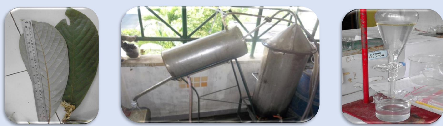
Fig. 1 Steam distillation of Actinodaphne glomerata leaf
