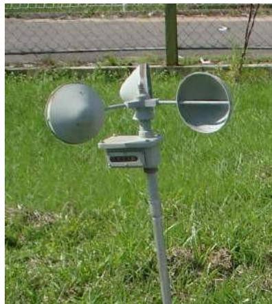
Gambar 3. Cup Counter Anemometer.
