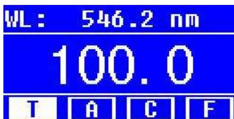
After 20 minutes' warm-up, the system goes into main interface. ( Fig.4-1) Press the key of **MODE** to change the functions.
